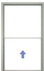
Window with one sliding section
