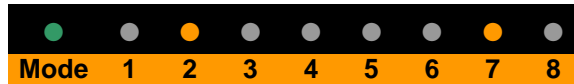
Figure 13: The sliding glass is moving in the closing direction after the alarm closing has been activated (see section 2.2)
