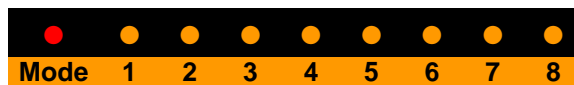
Figure 16: During power up the LEDs number 1 through 8 are lit one by one
