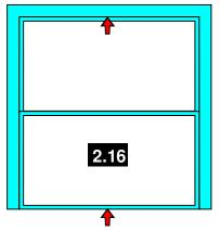
Tape the rubber strips on the top profile and beneath the sliding section. The rubber strips shall go along the whole width.
