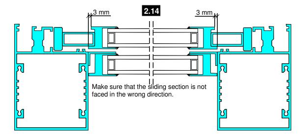
Replace the flat profiles to the side posts, the top profile and the bottom profile.
