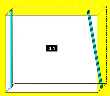
Fit the outer mounting strips (the mounting strips are not included in the delivery of the Sliding window).
