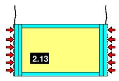
Fasten the sliding section to the runners. Section 2.14 shows in what direction the sliding section shall face.
