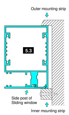
Example of mounting with angle strips and without screws on the outside.
