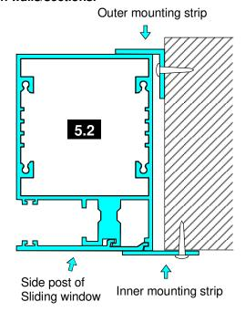
Example of mounting in a wall/section with fixed flange.
