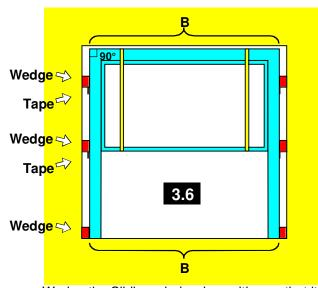
Wedge the Sliding window in position so that it will be at right angles. To make sure that the wedges will not drop down, place them above the pieces of tape on the side pillars.
