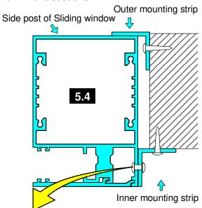
Note that no holes may be drilled in the Sliding window since electrical parts and moving parts are mounted in these sections. The angle strip must therefore be secured to the Sliding window by the manufacturer.
